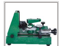
Inspect accuracy of test indicators
